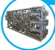
Gas seal panels, according to ISO 10438:2008 Part 4 and API 614 Fifth Edition Chapter 4, are designed to supply seal and buffer gas to the shaft seals. They include filters, controls, piping or tubing and the related instruments and cover a wide array of flows, pressures and material grades.
